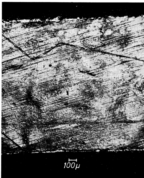
Fig. 3.5. Micrograph of the surface of annealed vanadium, specimen V2a. The edges are parallel to the current direction.
